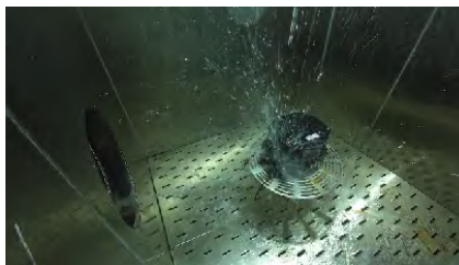
Length measurement sensor 48-hour rain test
