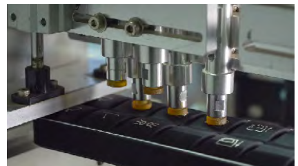
Panel buttons cycled 1.2 million times
