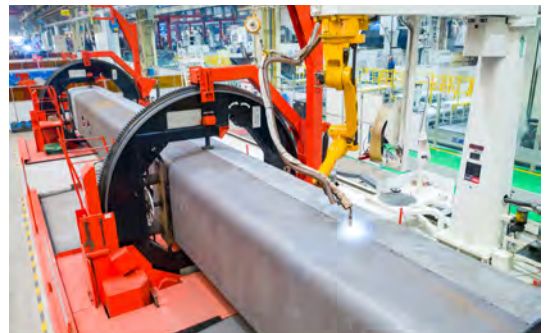
UNMANNED AUTOMATIC WELDING
