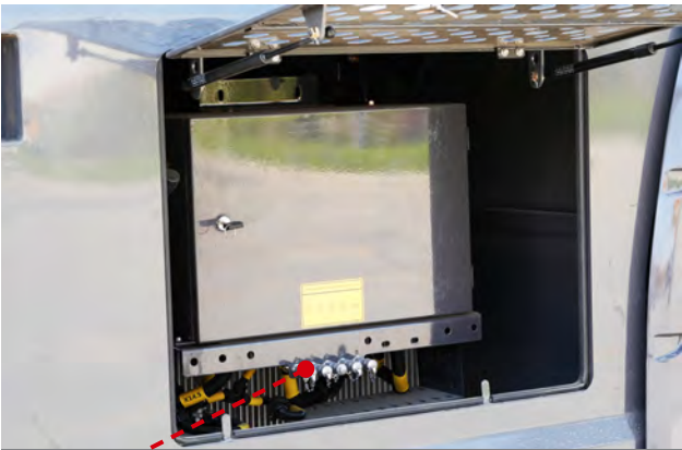
The pressure testing ports are centrally arranged.
