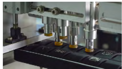
Panel buttons cycled 1.2 million times
