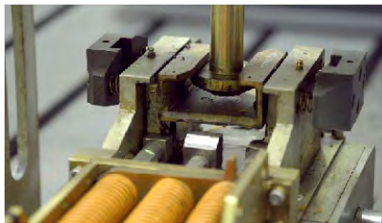
Telescoping mechanism Smoothness test
