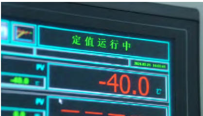
HMI display Low-temperature performance test under -40 °C
