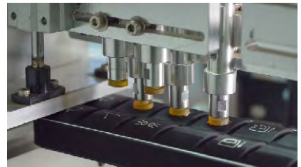
Panel buttons cycled 1.2 million times
