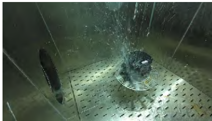
Length measurement sensor 48-hour rain test
